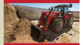
Loader mounting is fast and easy, thanks to our unique "Lock and Go" connection system. Our Euro style quick hitch system from ALO also allows for the easy interchange of bucket, bale spear, pallet fork and other tools.
