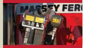
Loader hydraulic connections are conveniently located on the right side of the tractor for easy access. Flat face couplers ensure quick connection, and an available single lever system makes connecting the loader hydraulics fast and simple.
